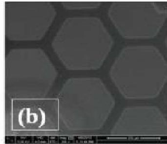
Junction of Ag/PCMO/NbSTO multilayer film grown by PLD and then covered with patterned. Ag pads
